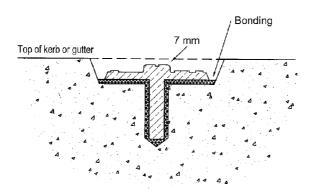
Fixation is by drilling and bonding with a suitable epoxy-resin compound
