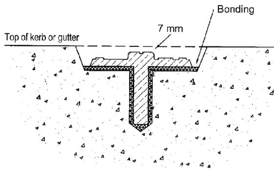
**Fixation is by drilling and bonding with a suitable epoxy-resin compound**
