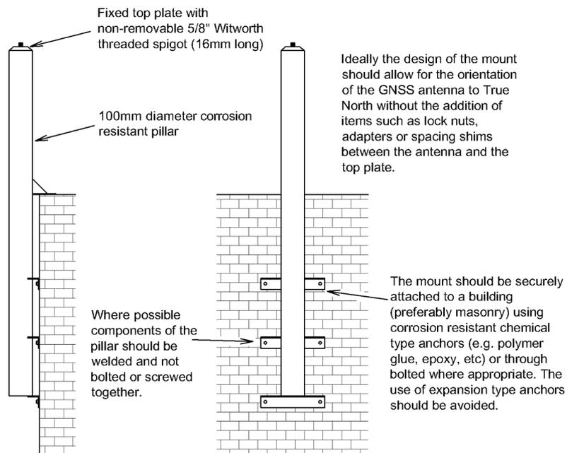
Note: Antenna mount type and dimensions vary according to constraints of the building.
