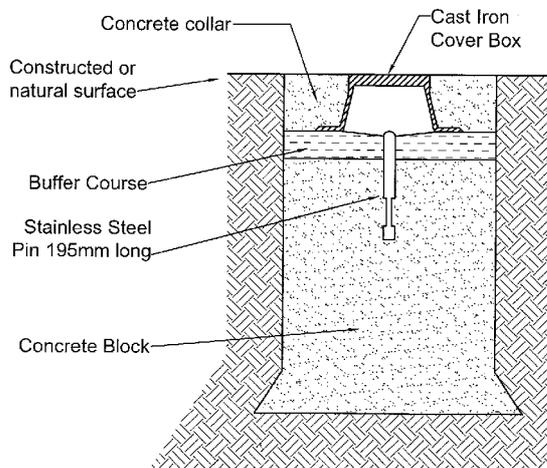
Minimum size of concrete 460mm deep by 380mm square and enlarged at the bottom. Where solid rock is met the depth may be varied.
